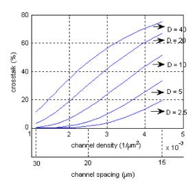
FIG. 8. Multichannel operation. The crosstalk is plotted as a function of channel spacing (and channel density) for different device diffusive constants D (in  $\mu \text{m}^2/\text{ps}$ ).
