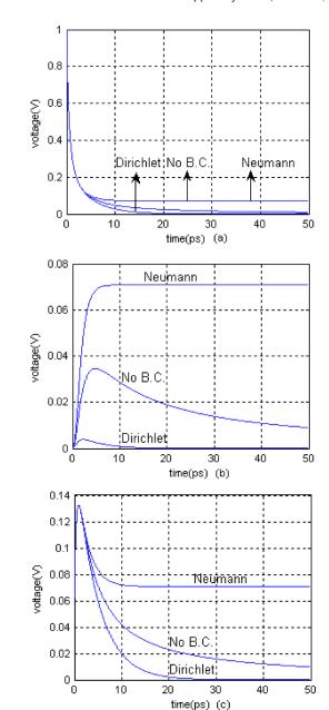
FIG. 3. Diffusive conductive voltage decay due to the three different boundary conditions (no boundary, V=0, and  $\nabla V=0$ ): (a) at the center of the switch, (b) at a point very near to the switch contact line, and (c) at the midpoint between the switch center and contact.
