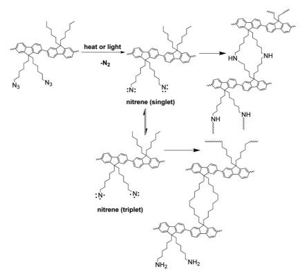
Scheme 1 Decomposition of azides under light or heat to produce nitrene which can be in singlet or triplet states. Each states react differently; singlet nitrene undergoes insertion while triplet (diradical) nitrene abstracts available protons by producing radicals which will combine with other radicals to form a cross-linked polymer.
