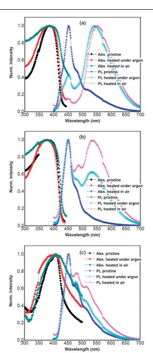
**Fig. 5** Normalized absorption and PL spectra of (a) PFA, (b) PFB and (c) PF annealed at 220 °C for 2 h under argon and in air.
