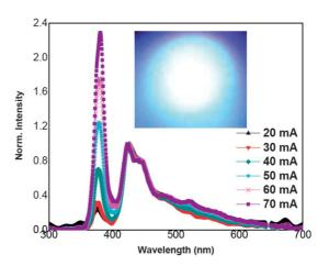
**Fig.** 7 Spectral behaviour of PFA hybridized on n-UV InGaN/GaN based LED at different current injection levels. The spectra are normalized according to the peak at 425 nm.
