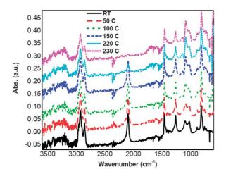
Fig. 4 In-situ FT-IR measurement of PFA under heat exposure.
