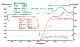
Fig. 3 DSC analyses of PFA and PFB. The exothermic peak of PFA centred at 218  $^{\circ}$ C indicates the cross-linking mechanisms taking place as highly reactive nitrene species insert into side chains or polymer backbone.
