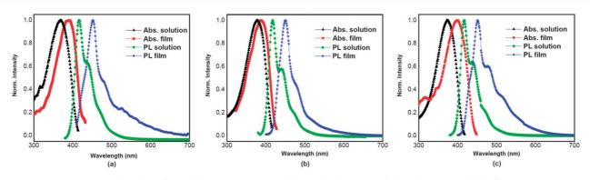
Fig. 2 The absorption and fluorescence spectra of (a) PFA, (b) PFB, and (c) PF in THF and thin film.
