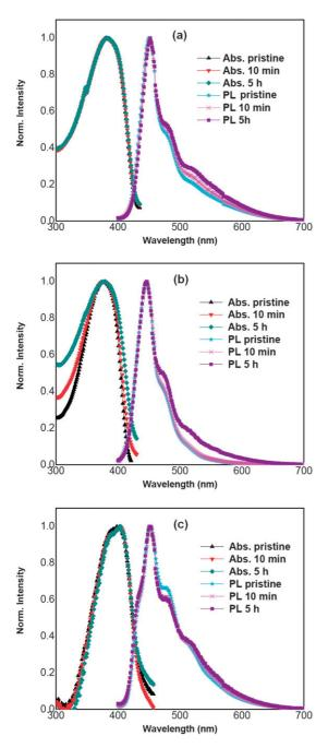
**Fig. 6** Determination of the spectral stability of (a) PFA, (b) PFB, and (c) PF after UV irradiation on n-UV LED operated at 0.9 mA at 10 V.
