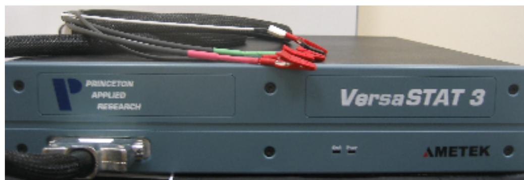
Figure 4.1.2 Our Versastat3 potentiostat/galvanostat.
