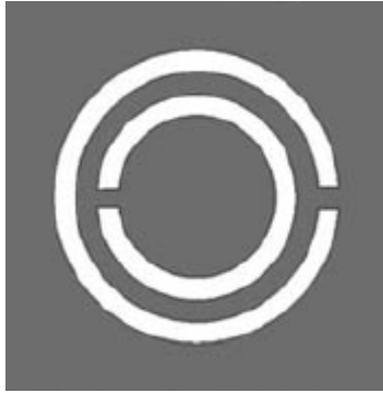
Figure 3.3 Complementary split ring resonator (CSRR).
