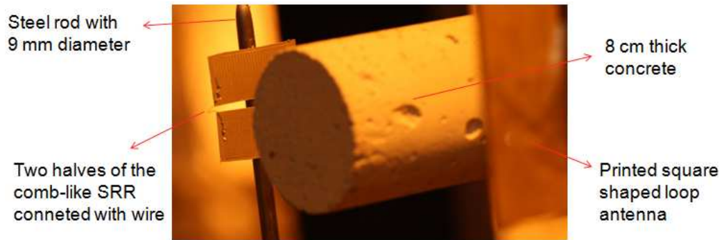
Figure 5.25 Full experimental setup with a concrete.
