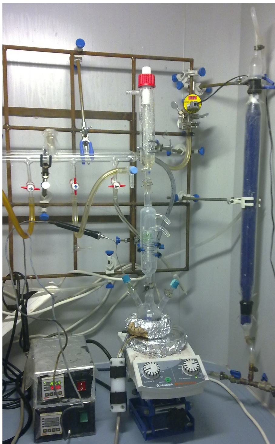
Figure 3.1: Our NPL synthesis setup in a fume hood consisting of a three neck flask, a temperature controller, a pressure gauge and a Schlenk line at our Bilkent UNAM laboratory.
