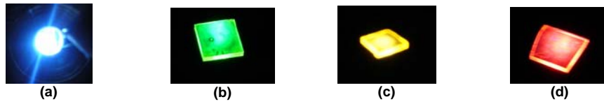
Figure 5.4.1.1. (a) Photograph of polyfluorene photoluminescence in blue. (b) the green NC film, (c) the yellow NC film, and (d) the red NC film.
