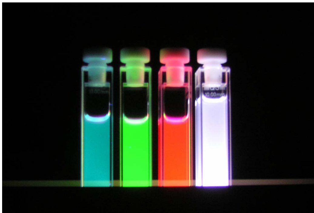
Figure 4.1.3. Photograph of cyan, green, and red CdSe core NCs and surface state emitting CdS NCs (from right to left).
