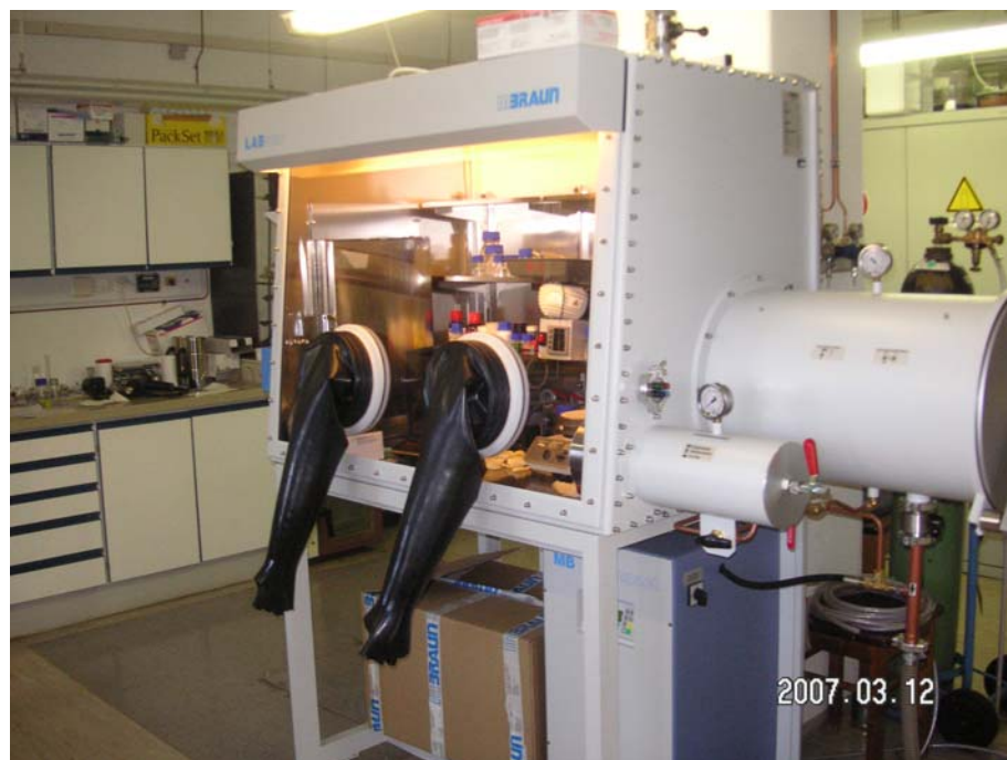
Figure 4.1.2. Photograph of glove box used for taking Se solution.
