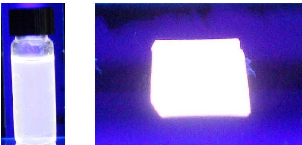
Figure 5.2.3. Photographs of white light emission from trap-rich CdS NCs in colloidal form (left) and in film form (right) under UV light illumination.
