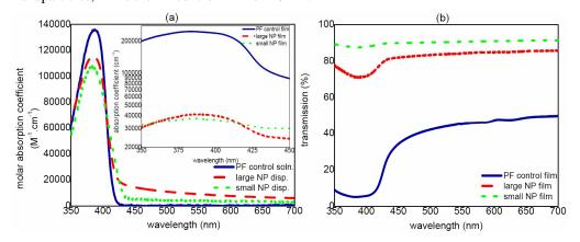
Fig. 2. Molar absorption coefficient of PF control solution and NP dispersions along with the absorption coefficient of PF control film and NP films in the inset (semi-logarithmic scale) and (b) transmittance spectra of PF control film and NP films.
