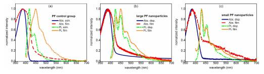
Fig. 1. Optical absorption and photoluminescence spectra of PF in different forms: (a) stock solution and polymer thin film as the control group, (b) large nanoparticle (LNP) dispersion and LNP film, and (c) small nanoparticle (SNP) dispersion and SNP film.
