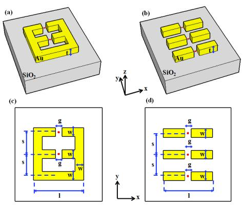
Fig. 1. Three-dimensional (3D) structures of (a) a comb-shaped nanoantenna with two teeth and (b) a three-dipole nanoantenna array, and their perspective views in (c) and (d), respectively, seen from constant z plane passing through the gap center points. In the figure red dots represent the gap center points.
