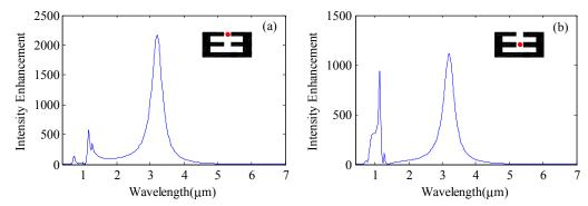
Fig. 4. Field intensity enhancement spectrum for two-teeth comb-shaped nanoantenna calculated at the center points of (a) the outer and (b) the inner gap. Here, the outer and inner gap centers are marked with red dots in the corresponding inner drawings.
