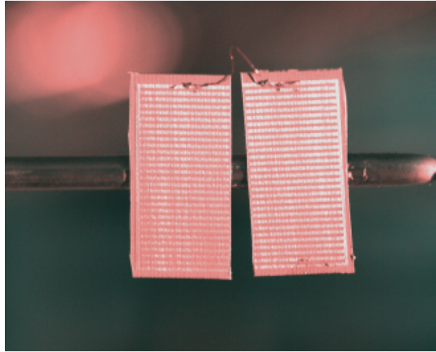
Figure 2.18: A possible misalignment where two NSRR probe parts on a rebar are rotated on the same plane.
