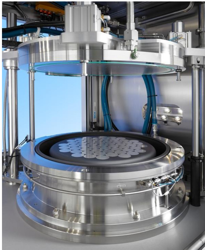
Figure 2. 2 CRIUS-II close coupled showerhead MOCVD reactor. A state of the art tool for high throughput GaN growth. After [14].
