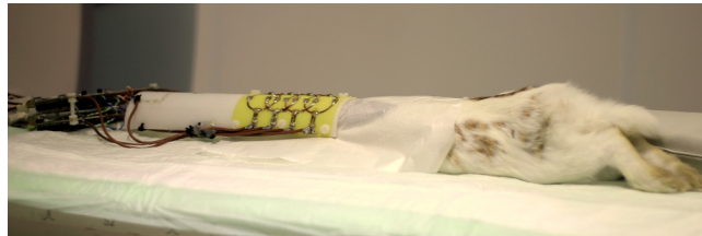
Figure 5.1: An eight-channel open surface coil system used for ex-vivo animal studies.
