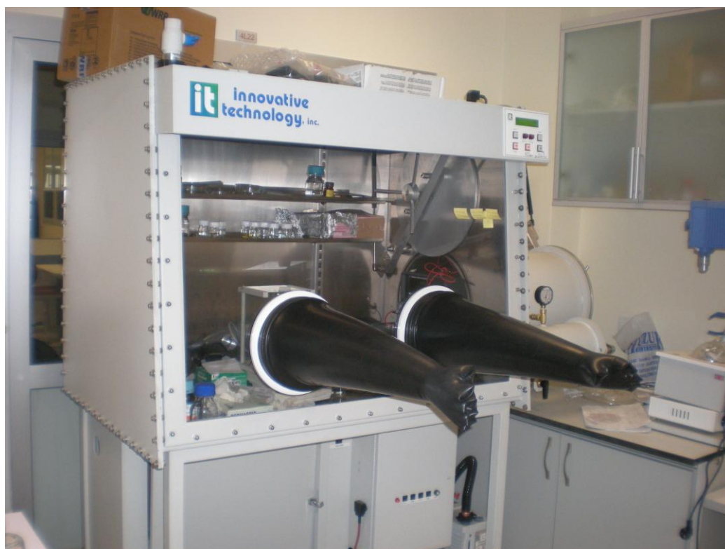
Figure 3.3.1.2 Photograph of glove box to work in oxygen-free environment.
