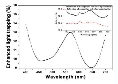
Figure S1. Increased light trapping of the nanopillar solar cells after the quantum dot hybridization, along with reflection spectra of the nanopillar cells before and after the hybridization shown in the inset.
