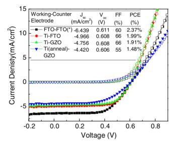
**Figure 3.** J-V characteristics of the bottom- and top-illuminated DSCs under illumination (filled symbols) and in the dark (open symbols). Devices are named in the format of working electrode–counter electrode. (\*) denotes the bottom-illuminated device.
