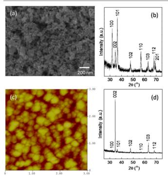
**Figure 1.** SEM image of ZnO porous film fabricated on Ti substrate (a) and its XRD pattern (b). AFM images of the GZO counter electrode deposited on glass substrate by MOCVD (the unit of scale bar is  $\mu$ m.) (c) and its XRD pattern (d).
