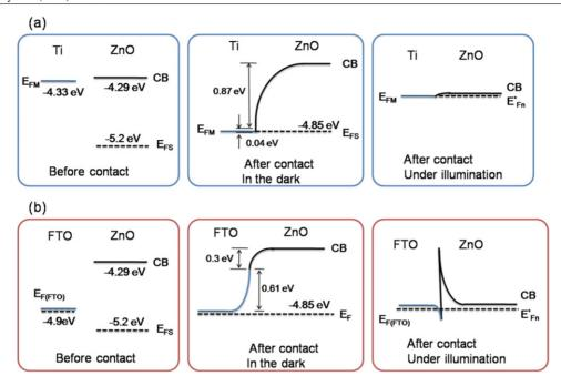
**Figure 6.** Schemes of electron energy at (a) Ti/ZnO contact and (b) FTO/ZnO contact. Left diagrams illustrate the energy level of individual layers before contact, centre ones show the band bending at the interface in the dark, and right diagrams show the formation of ohmic and Schottky contact for Ti/ZnO and FTO/ZnO, respectively, under strong illumination and open circuit conditions.
