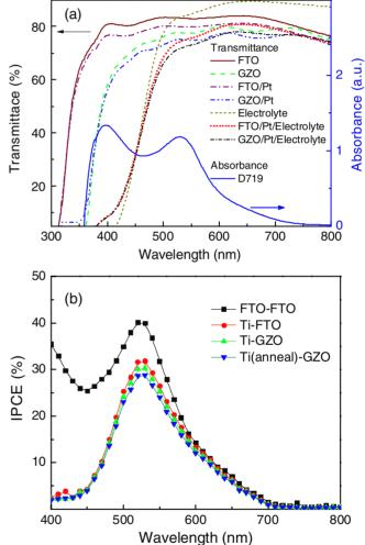
**Figure 4.** (a) Transmittance spectra of FTO and GZO with/without Pt and  $60 \mu$ m-thick electrolyte (left vertical axis) and absorption spectrum of D719 dye (right vertical axis). (b) IPCE spectra of the fabricated devices.
