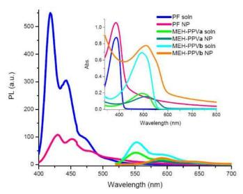
Fig. 3. Onset: Emission spectra of PF solution and its corresponding PF NP dispersion, MEH-PPVa solution and its corresponding MEH-PPVa NP dispersion, and MEH-PPVb solution and its corresponding MEH-PPVb NP dispersion. Inset: Absorption spectra of PF solution and PF NP dispersion, MEH-PPVa solution and MEH-PPVa NP dispersion, and MEH-PPVb solution and MEH-PPVb NP dispersion.
