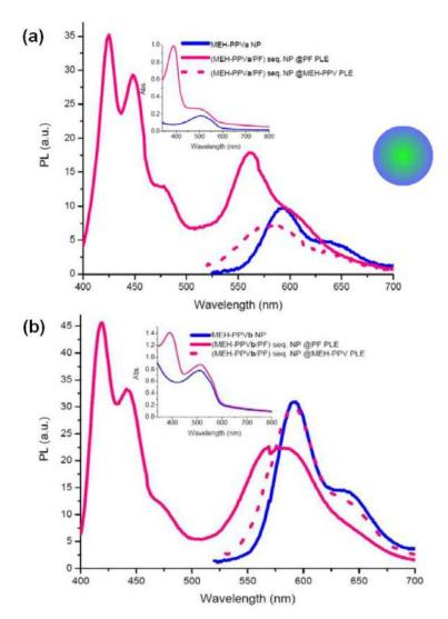
Fig. 9. a) Onset: Emission spectra of MEH-PPV NPs, (MEH-PPVa/PF) sequential NPs at absorption maximum of PF (solid) and MEH-PPV (dotted). Inset: Absorption spectra of MEH-PPV NPa and (MEH-PPVa/PF) sequential NPs, b) Onset: Emission spectra of MEH-PPVb NPs, (MEH-PPVb/PF) sequential NPs at absorption maximum of PF (solid) and MEH-PPV (dotted). Inset: Absorption spectra of MEH-PPVb NP and (MEH-PPVb/PF) sequential NPs.
