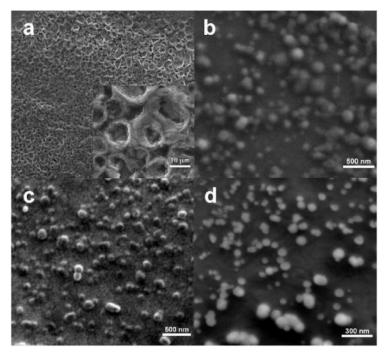
Fig. 2. SEM micrographs of films prepared from (a) PF solution, (b) PF NP dispersion (c) MEH-PPVa NP dispersion, and (d) (MEH-PPVa/PF) sequential NP dispersion. The last image is taken with a tilt angle of 15°.
