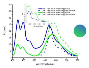
Fig. 6. Onset: Emission spectra of (PF + MEH-PPVa) and (PF + MEH-PPVb) mixed NPs at absorption maximum of PF (solid) and MEH-PPV (dotted). Inset: Corresponding absorption spectra of (PF + MEH-PPV) mixed NPs.
