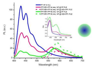
Fig. 7. Onset: Emission spectra of PF NPs, (PF/MEH-PPVa) sequential NPs at absorption maximum of PF (solid) and MEH-PPV (dotted), and (PF/MEH-PPVb) sequential NPs at absorption maximum of PF (solid) and MEH-PPV (dotted) Inset: Absorption spectra of PF NPs and (PF/MEH-PPV) sequential NPs.
