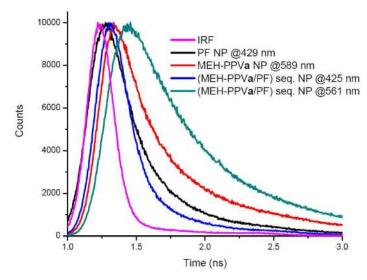
Fig. 10. Biexponentially fitted decay curves of PF NPs at 429 nm (0.26 ns), MEH-PPVa NPs at 589 nm (0.51 ns) and (MEH-PPVa/PF) sequential NPs at 425 nm (0.17 ns) and 561 nm (0.90 ns). Reported lifetimes are average intensity weighted values and decay fit parameter "R" ranges from 0.8 to 1.1.
