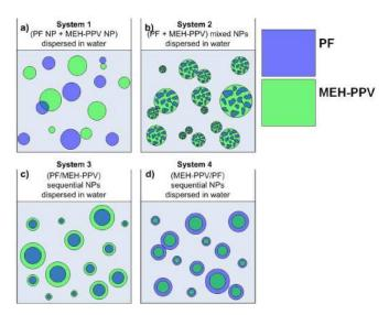
Fig. 1. Schematic representation of the proposed nanostructures for polymer nanoparticles formed from PF and MEH-PPV via the reprecipitation method. (a) System 1: (PF NP + MEH-PPV NP), (b) System 2: (PF + MEH-PPV) mixed NPs, (c) System 3: (PF/MEH-PPV) sequential NPs, and (d) System 4: (MEH-PPV/PF) sequential NPs.
