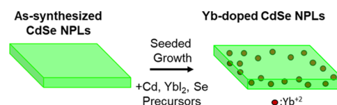
Figure 1. Schematic representation of the synthesis of Yb-doped CdSe NPLs.
